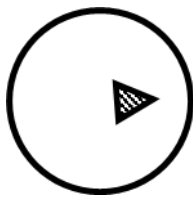
One way pump – fixed displacement
